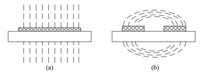
Figure 1: Two configurations for sensing proximity: (a) single electrode and (b) two in-plane electrodes.
