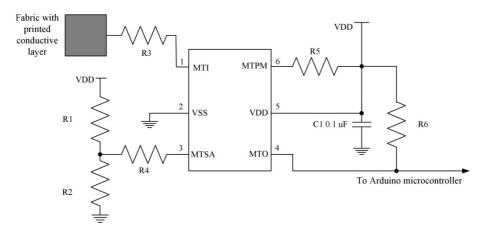
Figure 4: Circuit configuration using microchip proximity sensor IC.
