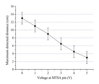
Figure 5: Maximum detected distance of the printed proximity sensor on polyester/cotton fabric.
